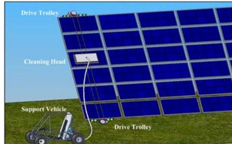
Figure 2: Concept of New Robotized Cleaner for Photovoltaic Panels.
