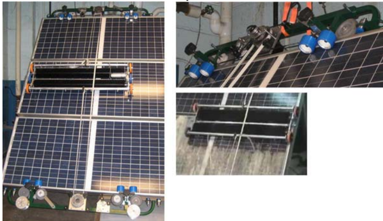
Figure 7: Prototype of PVCleaner Robot V1.0 and Close Up Views of the Trolley Carrier and Cleaning Head.
