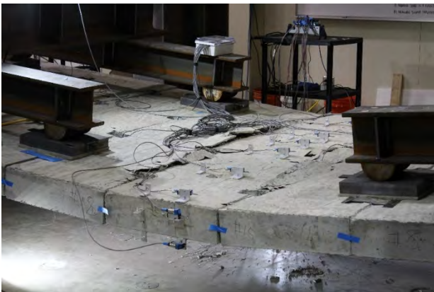
Fig. 13 – Concrete crushing between planks
