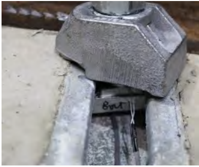
Fig. 9 – Large rotation of M20 clamp
