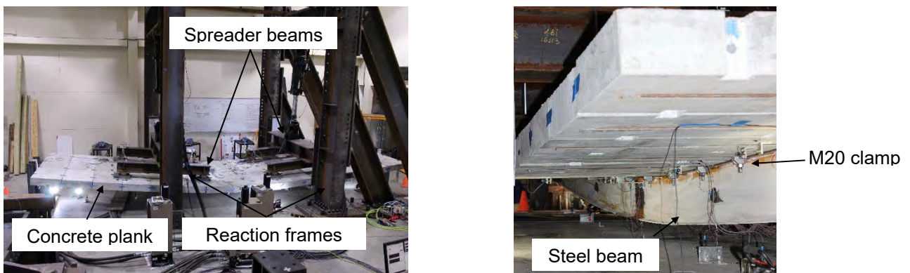
Fig. 11 – Composite beam test setup
