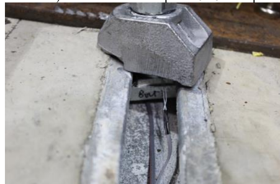
d) Complete disengagement of Clamp 3 at 2.56 in. slip
