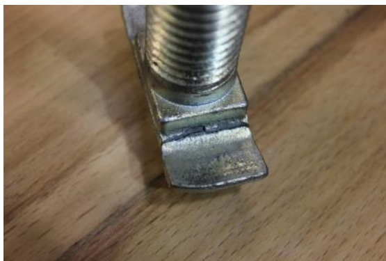
a) Head fracture in Bolt 4
