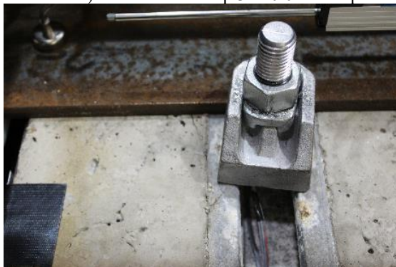
c) Rotation of Clamp 4 at 0.32 in. slip
