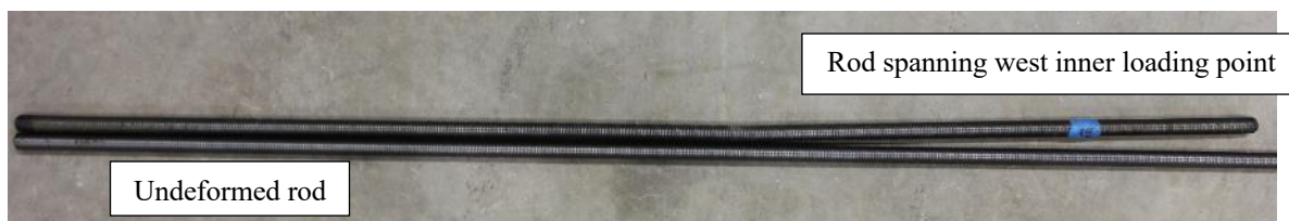
Figure 5.72 Deformation of fully threaded rod in Test 1-M24-2C-RH
