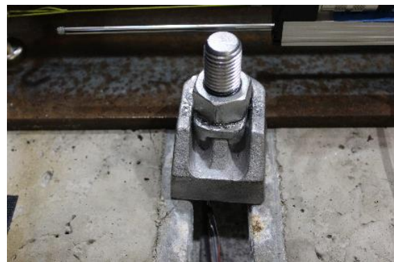
b) Rotation of Clamp 4 at 0.16 in. slip
