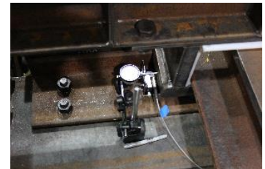
linear potentiometer at northwestern corner
