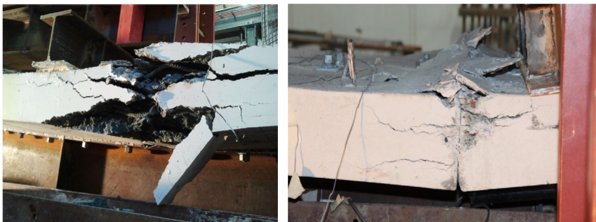
a) CB1 b) CB 2 Figure 5.46 Concrete crushing in different composite beam specimens [after (Ataei et al. 2016)]
