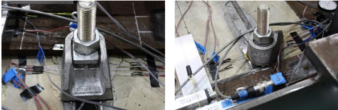
a) Rotation of Clamp 2 at 0.64 in. slip
