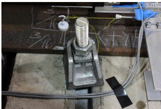
a) Rotation of Clamp 1 at 1.28 in. slip
