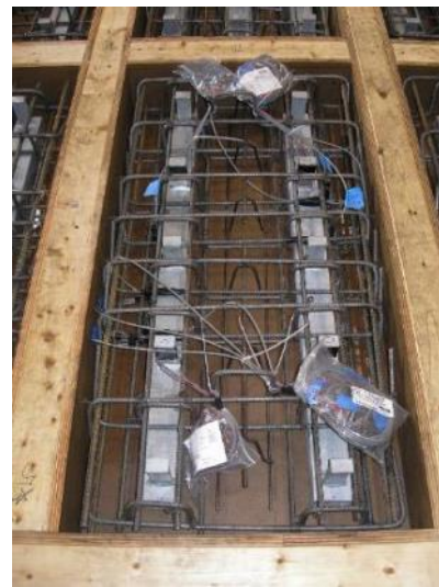
b) Heavy reinforcement pattern
