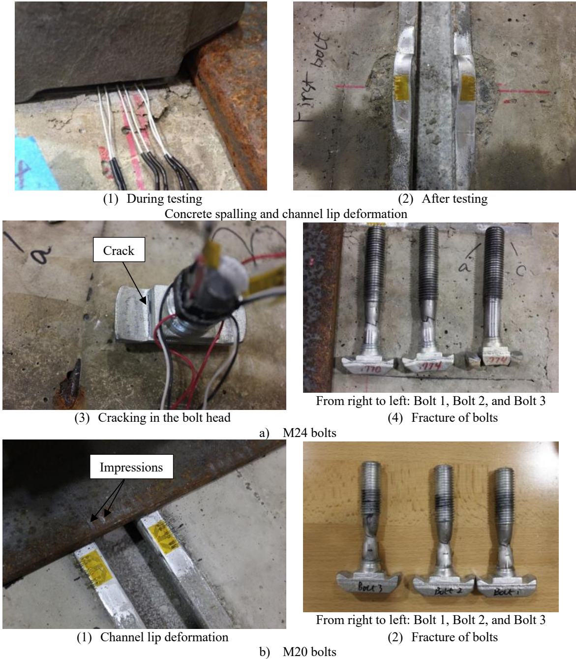
Figure 4.14 Photographs of bolt pretension tests
