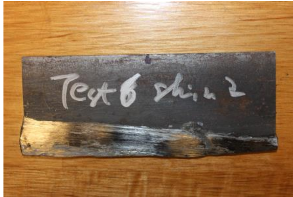
Scraped steel shim
