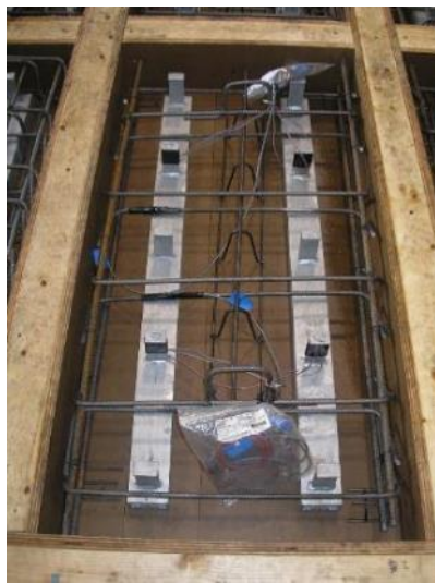
a) Light reinforcement pattern
