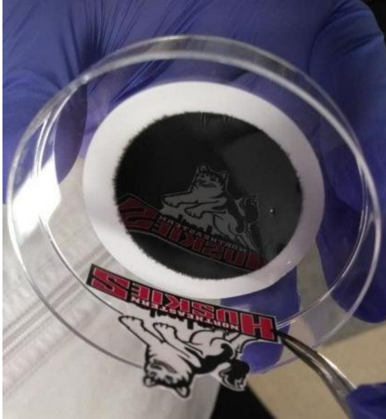
Supplementary Figure 10. clear "Huskies" picture could be reflected on MoS 2 -S film.
