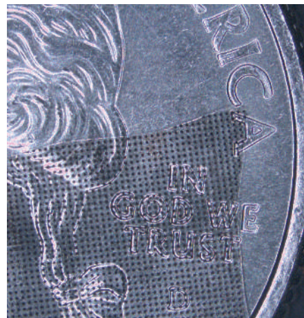
Figure 1 | Flexible friend. Jung and colleagues 6 nanotube-polymer composite, with its evenly spaced carbon pillars clearly visible.
