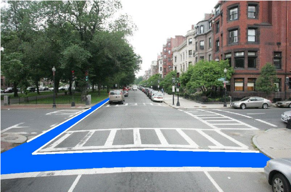
This figure shows a rendering of a bike box on Commonwealth Avenue. Note the painted bike lane extending across Gloucester Street to alert drivers of cyclist travel on the left.
