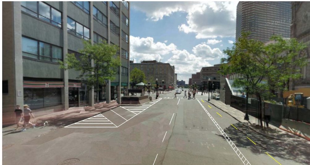
Figure 6.10: Rendition of R-A parking at bulbout at Dartmouth St. and Boylston St. note cross section changes from 35' to 44'
