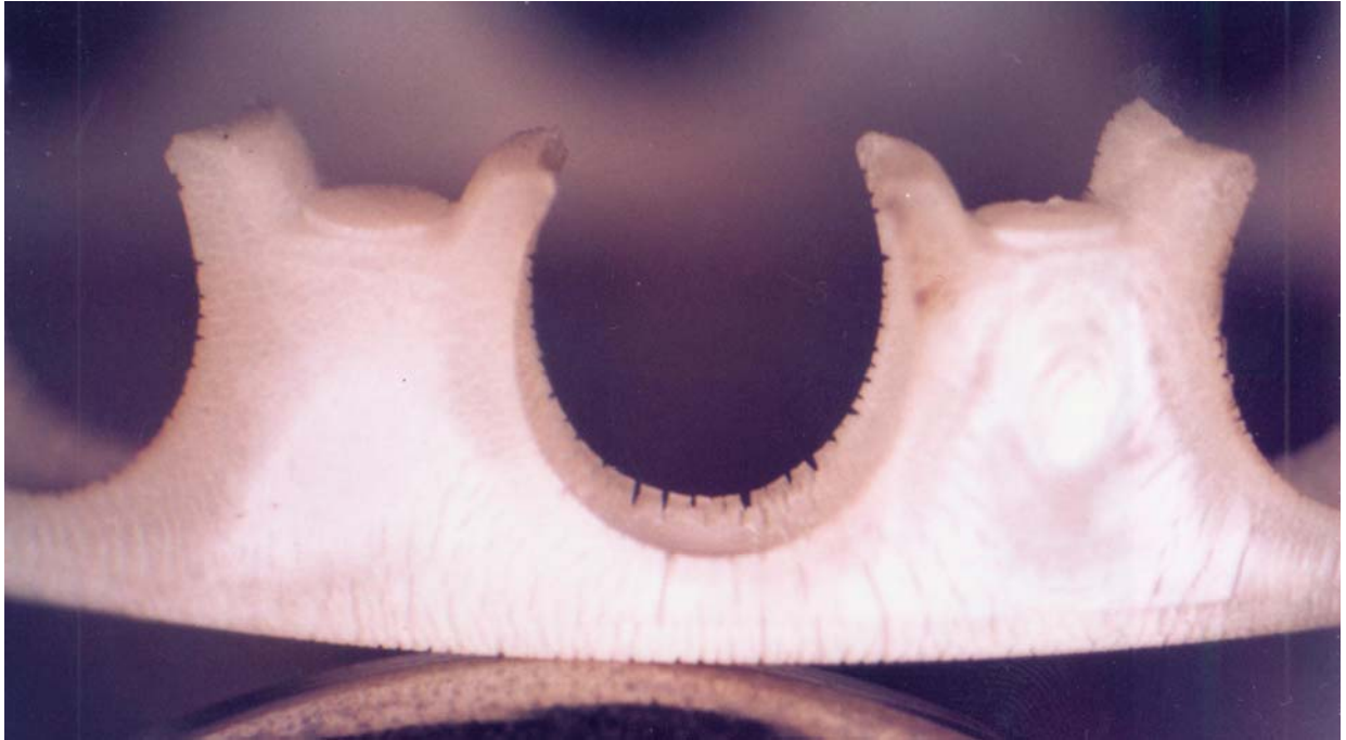
Figure 1: PEEK retainer after 10 years of storage.
