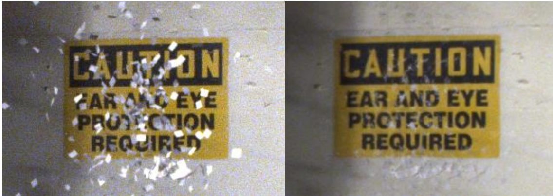
Figure 48. Light field based occlusion removal. The left is a raw image from one camera of an occluded sign. The right is a rendered using a light field array and median ray color selection.
