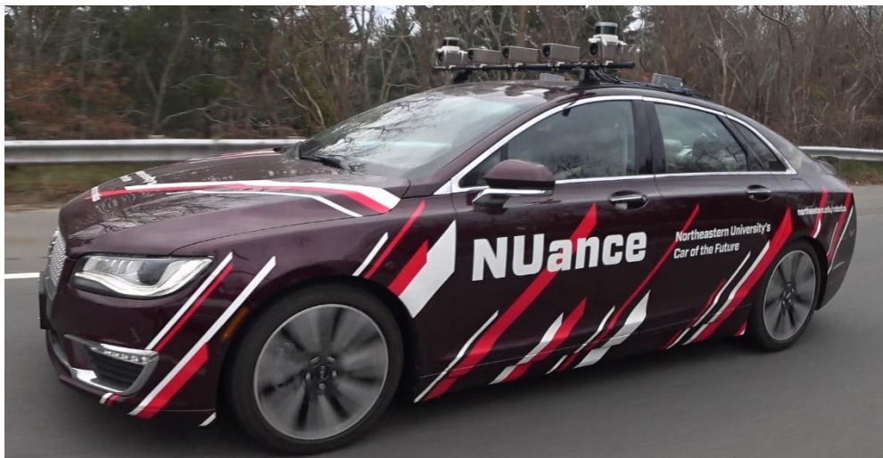
Figure 6. Northeastern University's Autonomous Car. A Lincoln MKZ with an ADAS kit modified by DataSpeed Inc.
